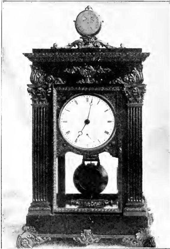
FIG. 476.—Breguet's Synchronizer.
